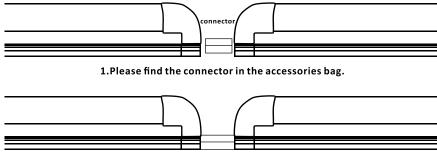
2. Plug the connector into the tube.
