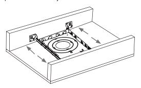
2.Place the J-box on the new structural plate and fix it by bending the clip.
