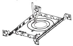
3.Place the plate between applicable joists where downlight will be installed; use a hammer to knock plate brackets into joists.
